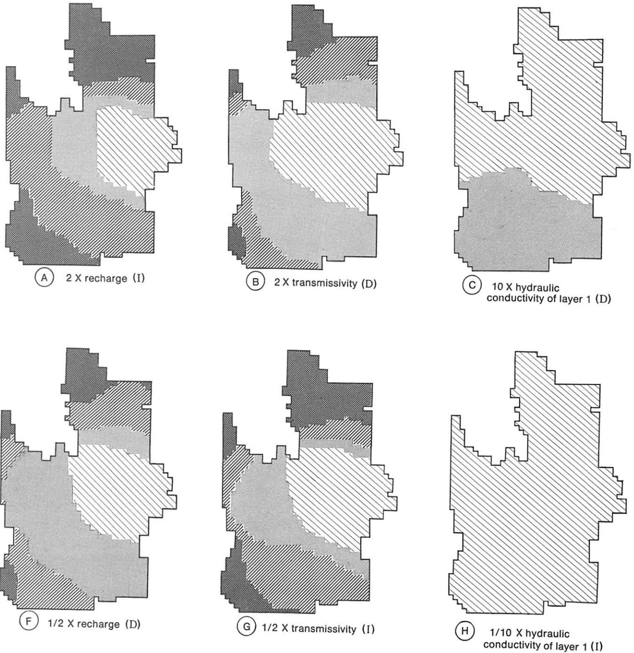
**Figure 25.** Sensitivity of model-simulated hydraulic heads in layer 2 to changes in natural recharge, transmissivity, hydraulic conductivity of layer 1, maximum evapotranspiration rate, and leakage during steady-state conditions.
