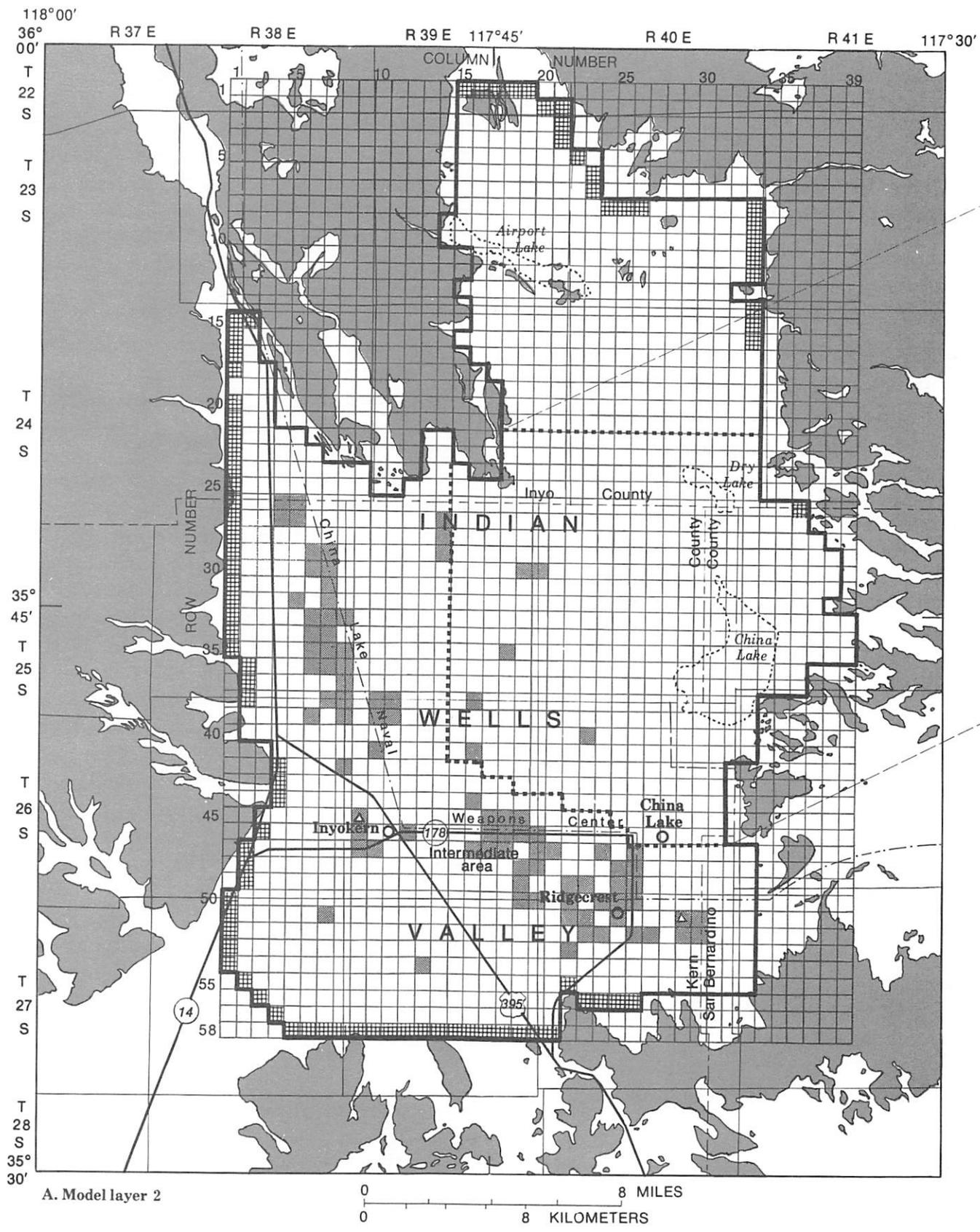
Figure 11. Grid network and areal distribution of recharge and discharge blocks for model layers 1 and 2.
