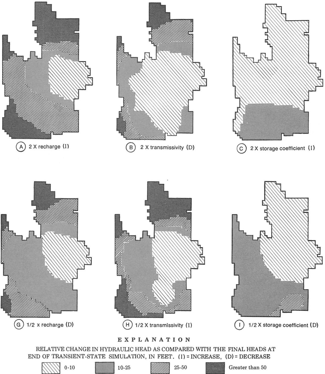
**Figure 26.** Sensitivity of model-simulated hydraulic heads in layer 2 to changes in natural recharge, transmissivity, hydraulic conductivity of layer 1, maximum evapotranspiration rate, and leakance at the end of transient-state simulation.
