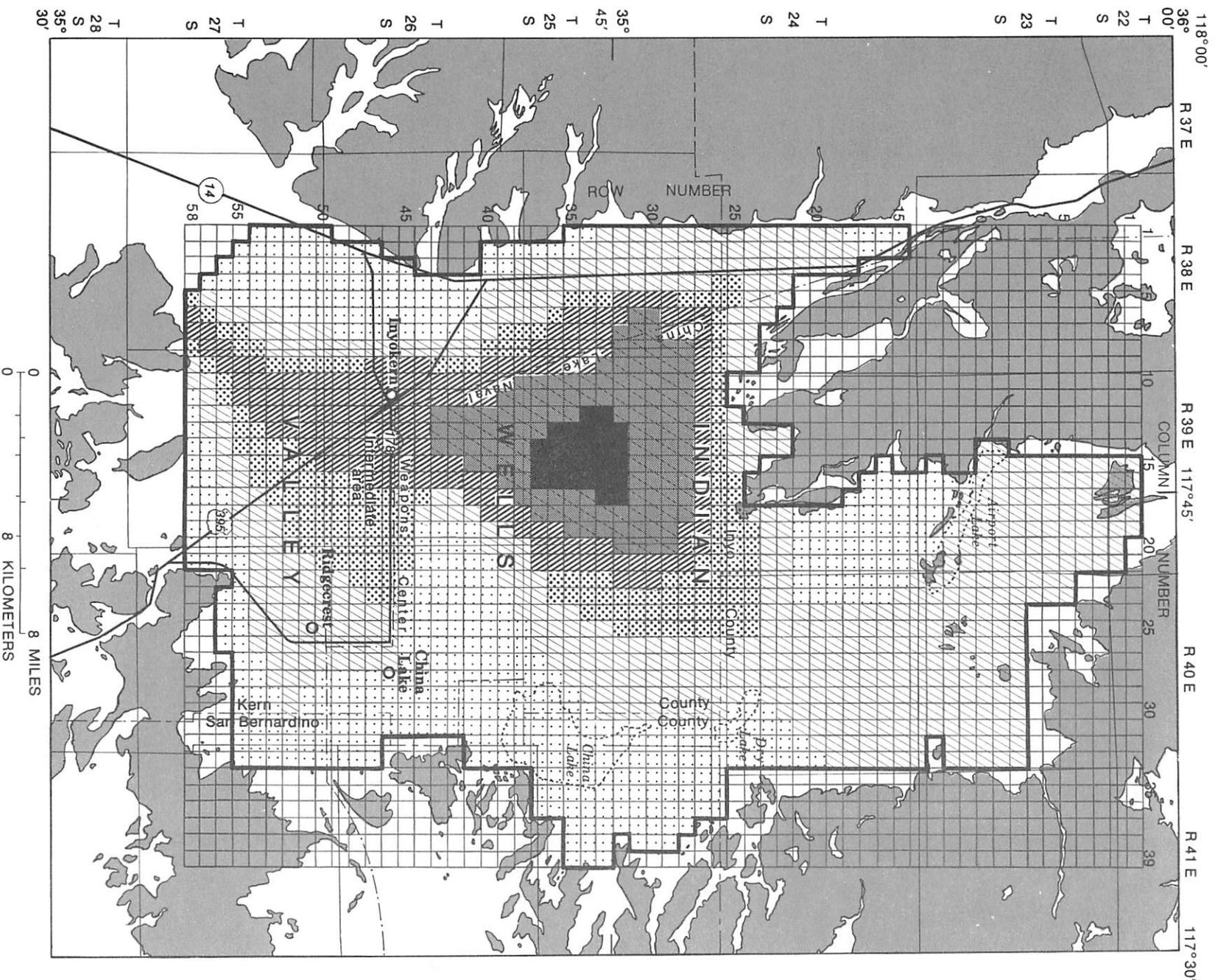
Figure 14. Areal distribution of transmissivity of layer 2, as simulated in the model.
