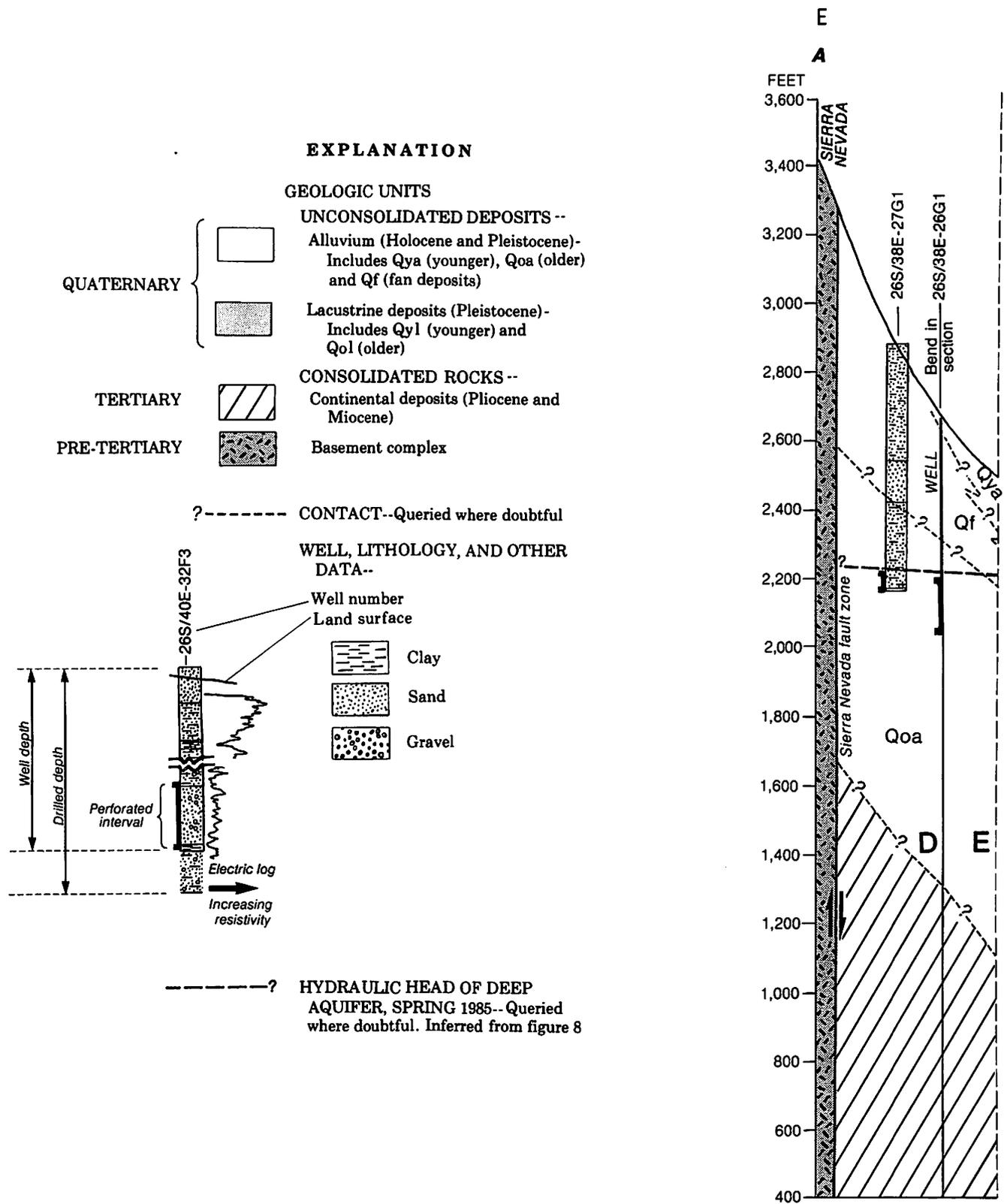
Figure 4. Diagrammatic geologic sections of the Indian Wells Valley ground-water basin.
