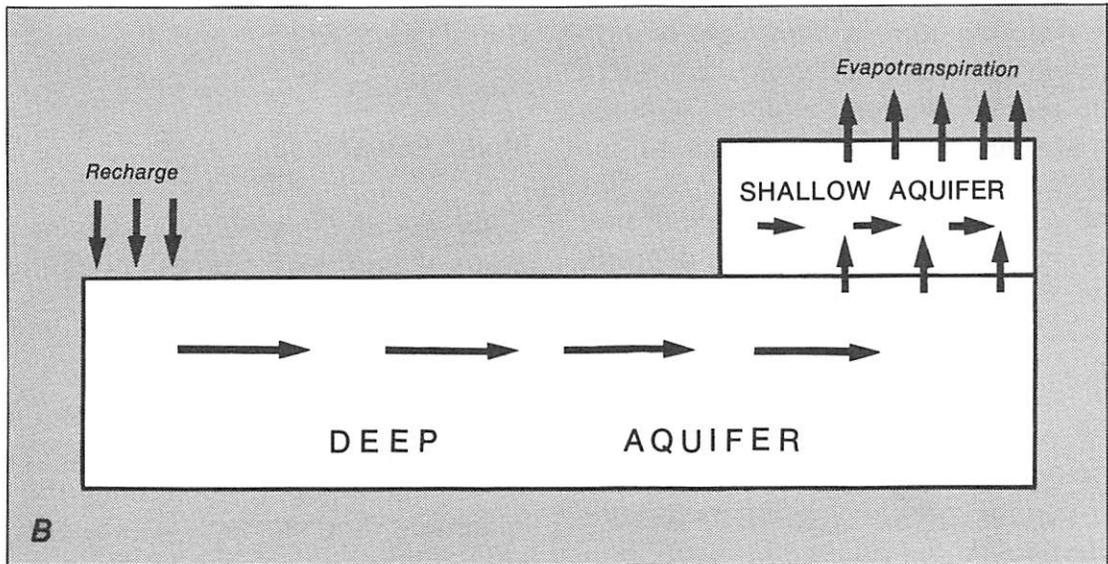
**Figure 10.** Conceptualization of the ground-water flow system in Indian Wells Valley. Arrows show direction of ground-water movement. *A*, Annotated diagrammatic section. *B*, Idealized ground-water movement.
