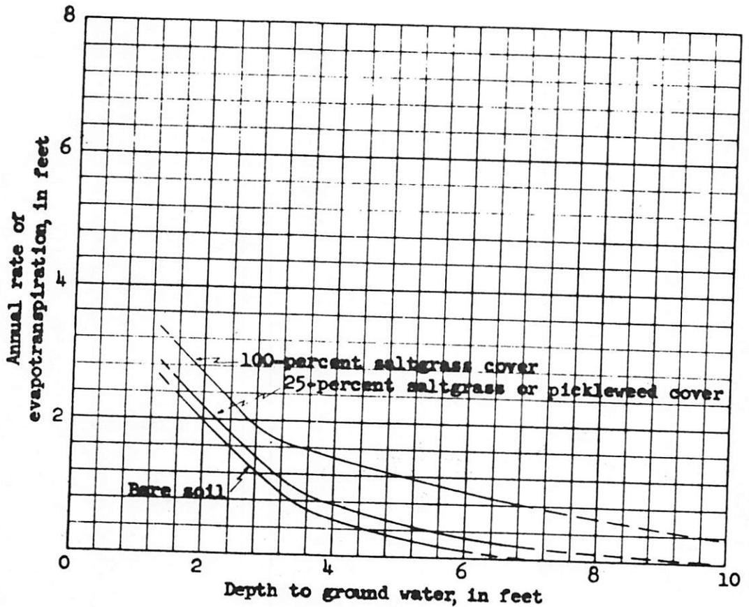
FIGURE 12.-- Relation of evapotranspiration to depth of ground water in Indian Wells Valley, California.
