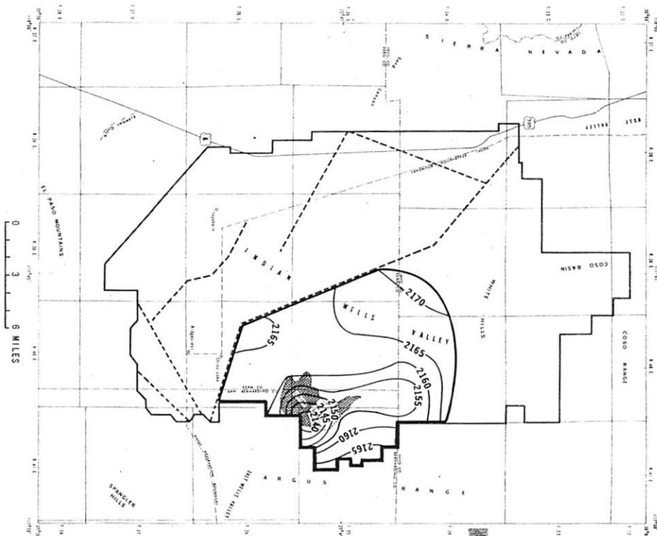
Figure 11. Model estimated steady-state water level contours for shallow aquifer.
