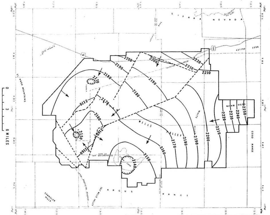
**FIGURE 1. Ground-water model boundary and water-level contours for deep aquifer.**
