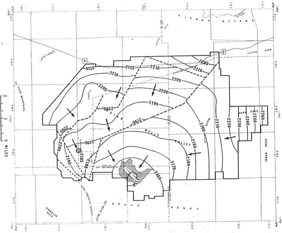
Figure 15. Water-level contours for deep aquifer, 1955
