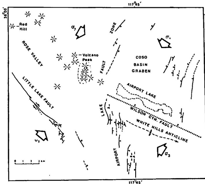
FIGURE 53. Schematic Diagram of the Southern Coso Range Showing the Local Stress Orientation.  $\sigma_3$  is the direction of least compressive stress, and  $\sigma_1$  is the direction of maximum compressive stress. The star symbols are cinder cones. The cones enclosed by a dashed line are the same age and composition.
