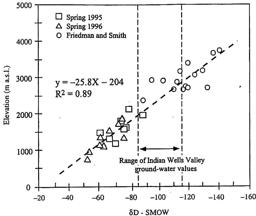
Figure 10. Plot of hydrogen isotope ratios ( $\delta D$ ) (SMOW, standard mean ocean water) versus elevation for the study area. Dashed line shows the linear regression for the data (equation shown). The data are from the rain gauge samples and published values (Friedman and Smith, 1972).
