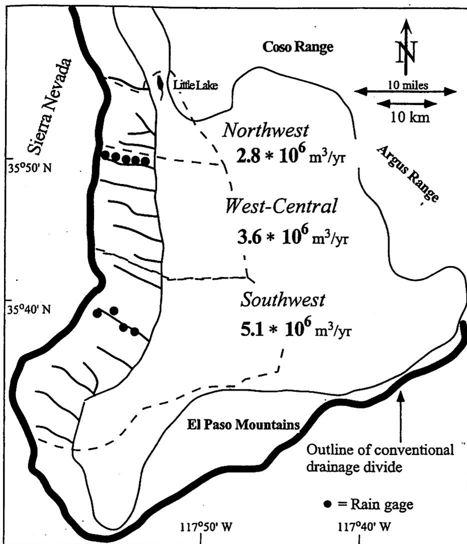
Figure 4. Results of recharge calculated by the precipitation-based method. The three sections of the study area and locations of the rain gauges are also shown. The value for the northwest section includes the contribution from the Little Lake stream outflow ( $1.6 \times 10^6 \text{ m}^3/\text{yr}$ ).
