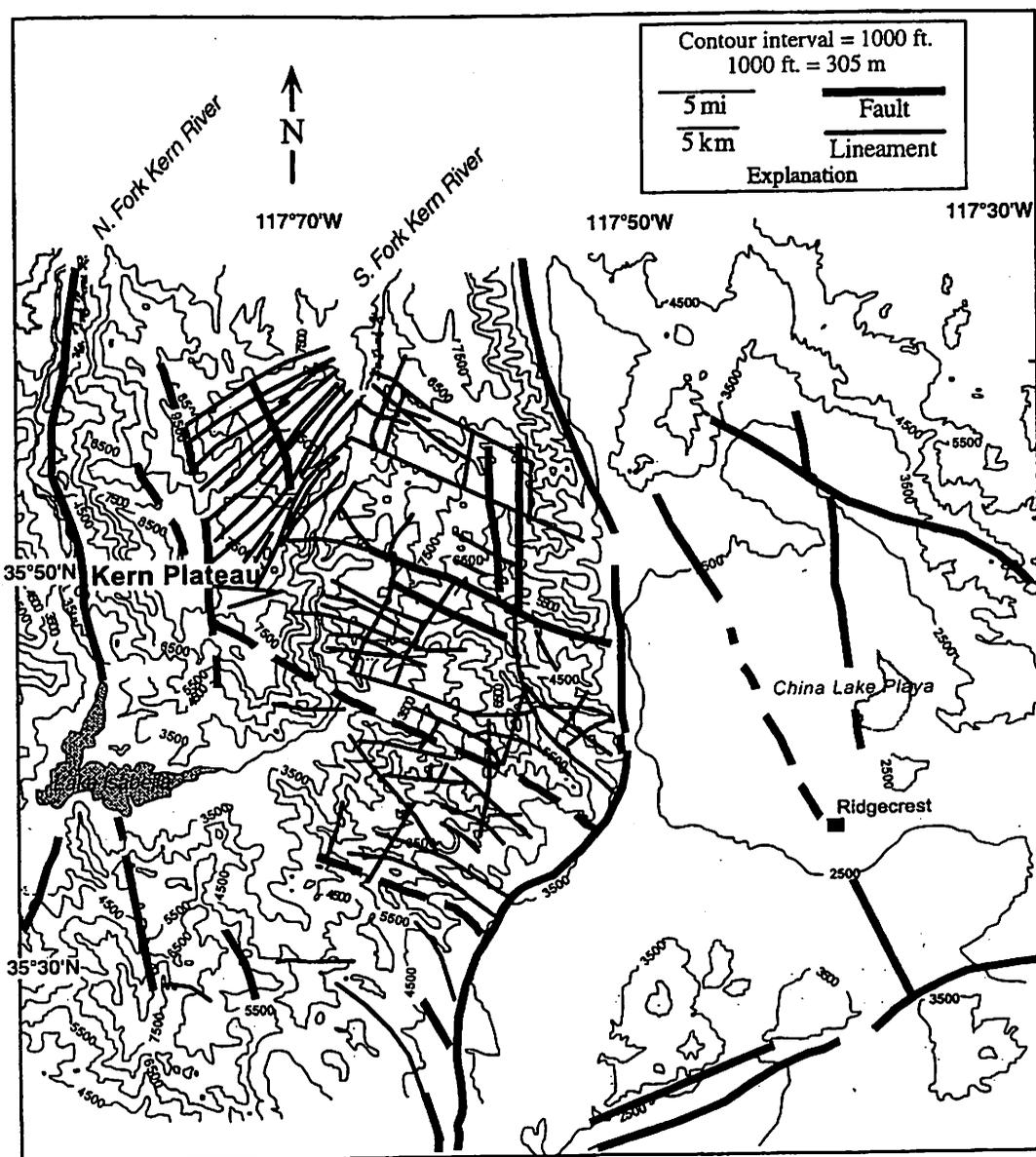
Figure 12. Map view of selected faults and lineaments in the study area. Modified from Ostdick (1997) and Figure 1 (this study).
