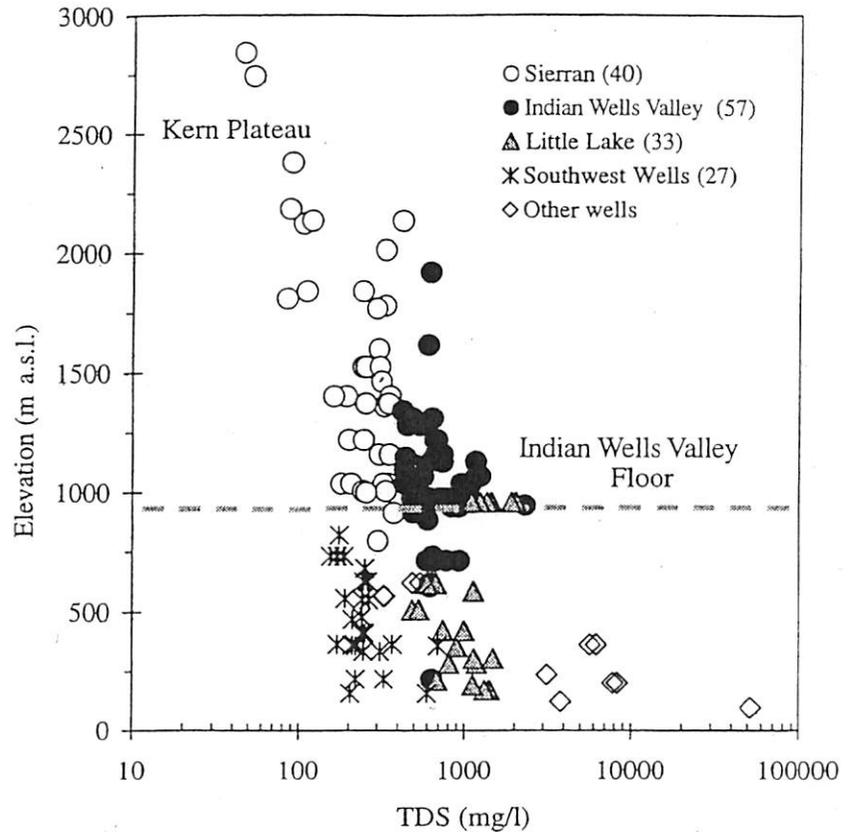
**Figure 9.** Plot of elevation (meters above sea level, m a.s.l.) versus total dissolved solids (TDS) for the hydrochemical facies and the deep wells (other wells) influenced by geothermal brine.
