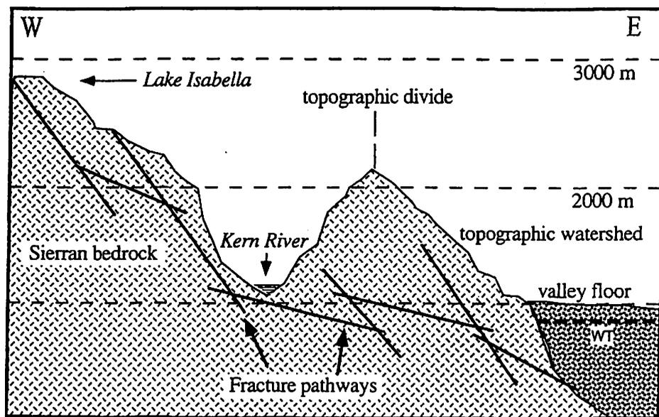
Figure 13. Conceptual model of fracture flow from the Kern Plateau into the Indian Wells Valley (not to scale). Flow crosses the local phreatic divide (Kern River) to discharge into the alluvial aquifer. WT—water table.
