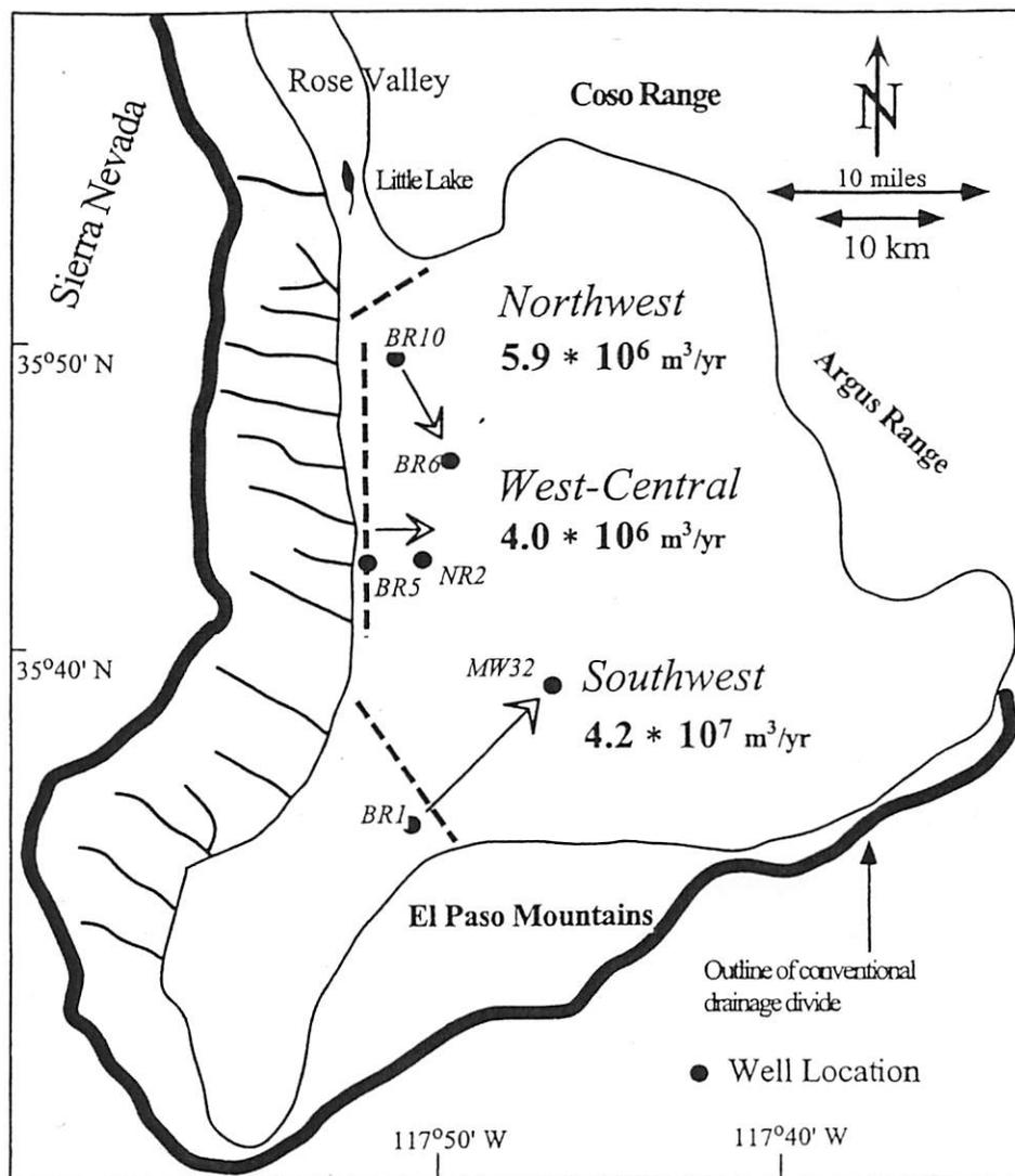
**Figure 5.** Results of the aquifer flux calculations using Darcy's Law. Data used in the calculations are listed in Table 1. The locations of the wells used to estimate the potentiometric gradient are shown with arrows to indicate the direction of flow. The heavy dashed lines indicate the cross-sectional area used to calculate the flux.
