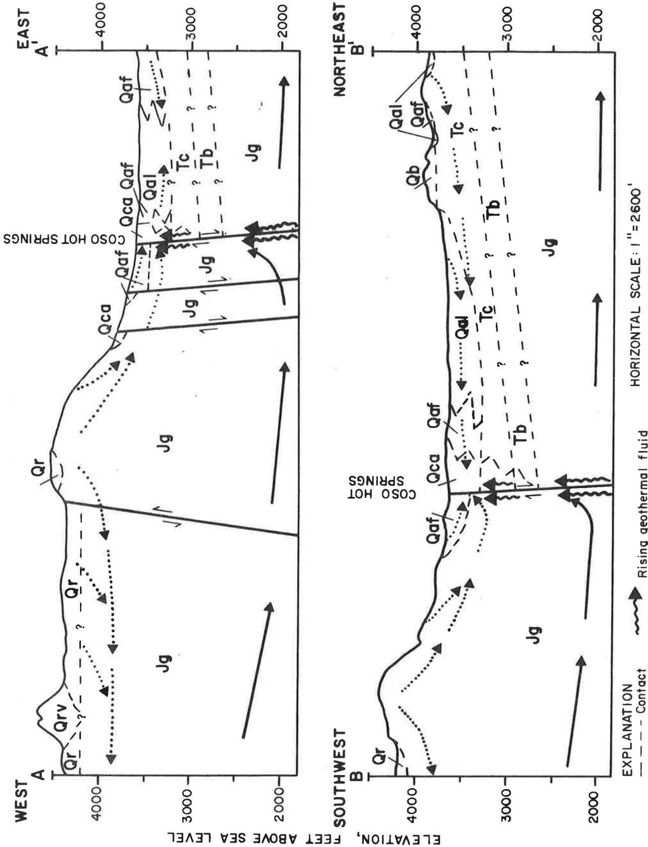
Figure 3. Interpretive Hydrogeologic Cross Sections, Coso Hot Springs and Vicinity.
